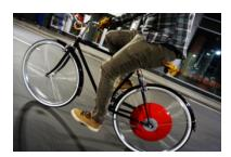
The Copenhagen Wheel has a rechargeable battery within the hub and a motor that is then operated by the battery. The wheel replaces the back wheel on a bike and is controlled by the bicyclist's smart phone. As the bicyclist pedals and brakes, energy is saved that can be used if climbing a hill or carrying heavier loads. The wheel is also smart and patterns your pedaling revolutions, learning how you pedal to give you the most seamless boost when needed.
