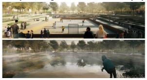
rink or ballfield). During a flood, the water would be held there but eventually sink into the ground or, on a gentle grade, return to the adjacent river. Designers in Copenhagen have expanded on the simple principle and designed parks that capture rain water with umbrellas and hold water in flexible panels on which children can jump. If integrated with a cycle track, the cycle track could be placed on higher ground around the flood prone area so the cycle track was always
